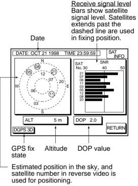
To return to the normal navigation data display, press the soft key RETURN.
